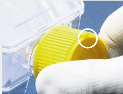
«VENT»-position 12 o'clock = gas exchange
